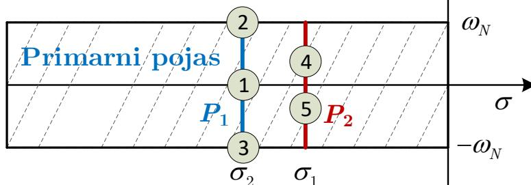
$$s = -\sigma_1 + j\omega \mid \omega \in [-\omega_N, -\omega_N] \rightarrow z = e^{-\sigma_1 T} e^{j\omega T}$$
